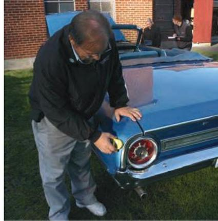
*Using a meter to check for filler and paint thickness during a pre-purchase inspection.*
